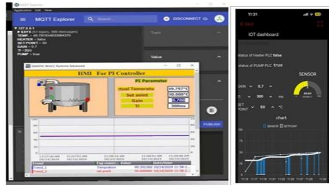
Figure 5. Multi-Interface Monitoring (MQTT Explorer, Simatic WINCC HMI, and mobile dash board)
