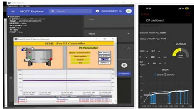
Figure 5. Multi-Interface Monitoring (MQTT Explorer, Simatic WINCC HMI, and mobile dash board)
