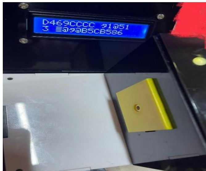
Figure 5. Arduino-based Li-Fi receiver circuit.
