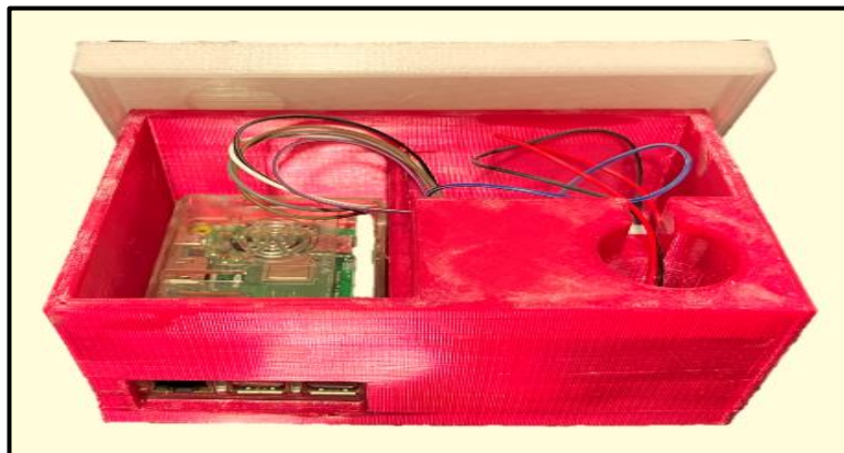
Figure 5. Geophone Electrical Circuit Setup; Custom-designed 3D-printed Case for the Geophone System
