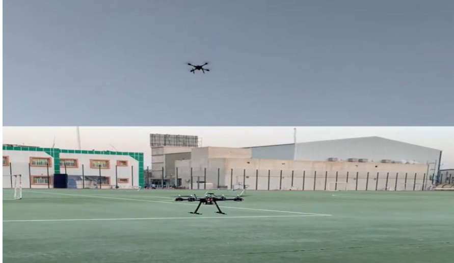
Figure 7 Flight mode evaluation using Position Hold (PosHold), demonstrating autonomous position stabilization during hover.
