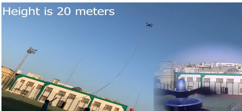
Figure 8. Maximum altitude test demonstrating stable ascent and hover at a height of 20 m.
