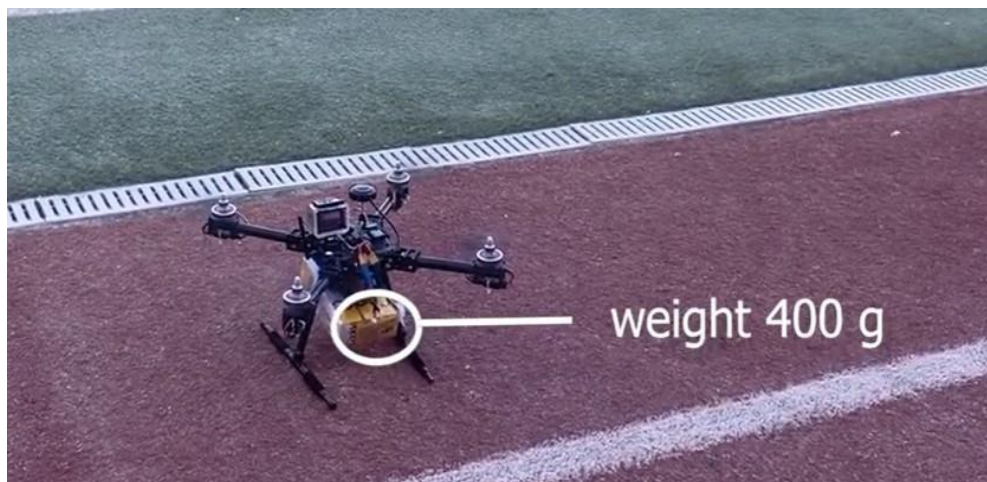
Figure 6. Payload-induced disturbance test with an additional 400 g mass attached to the quadcopter.
