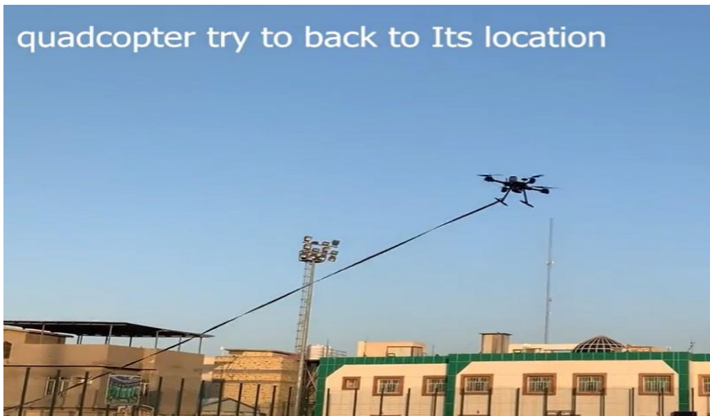
Figure 5. External disturbance rejection test by applying a sudden force through rope pulling during hover.
