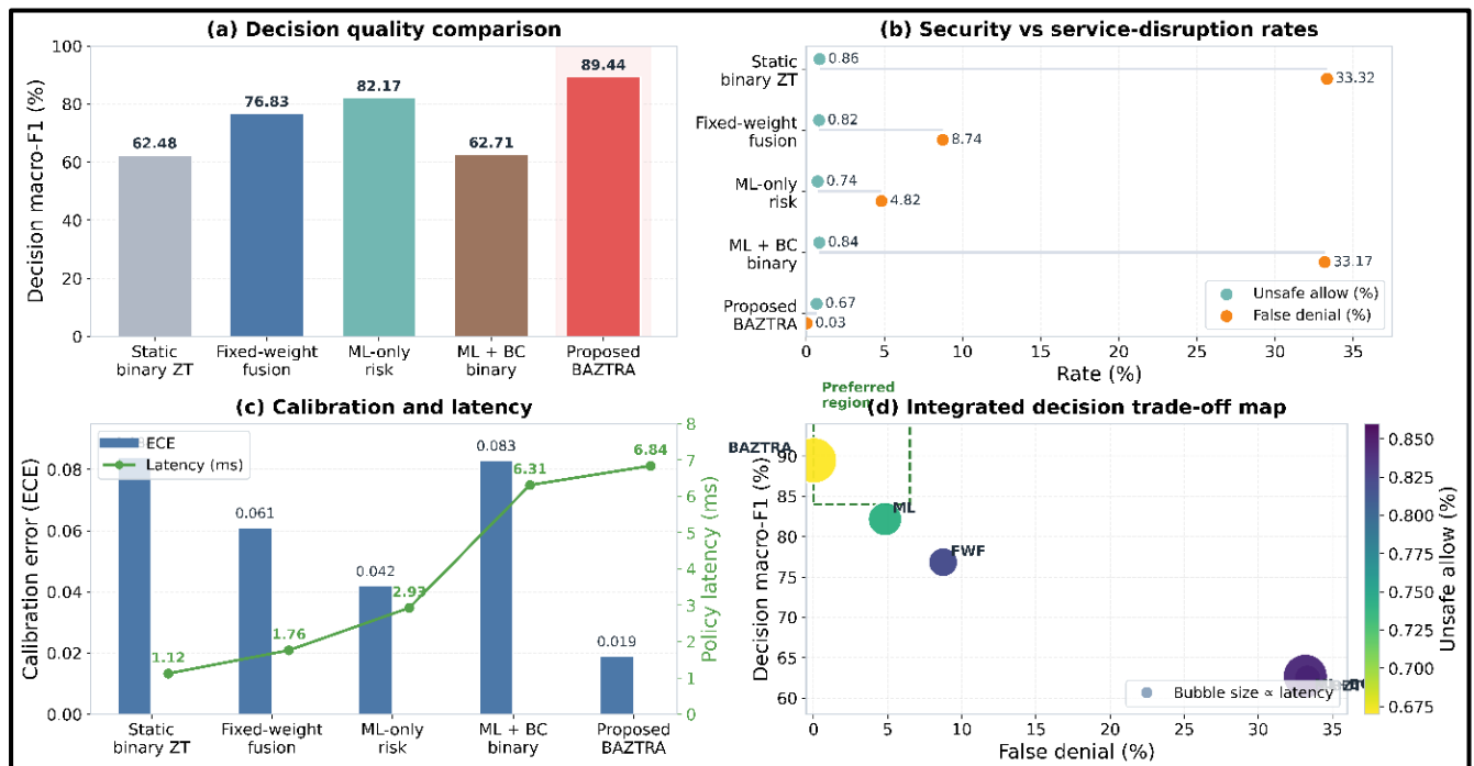
Figure 6. Comparative decision macro-F1, unsafe-allow rate, false-denial rate, calibration error, and latency of BAZTRA and the framework-level baselines.
